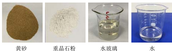
图 3 围岩相似材料 Fig.3 Surrounding rock similar materials
