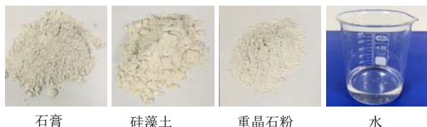
图 2 衬砌相似材料 Fig.2 Lining similar materials
