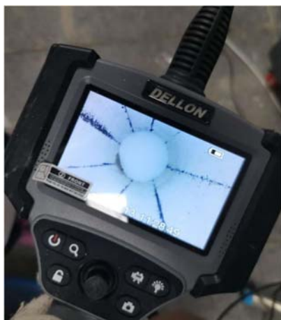
图 7 通过工业内窥镜对隧洞内部形态的监测 Fig.7 Observation of tunnel internal shape through industrial endoscope
